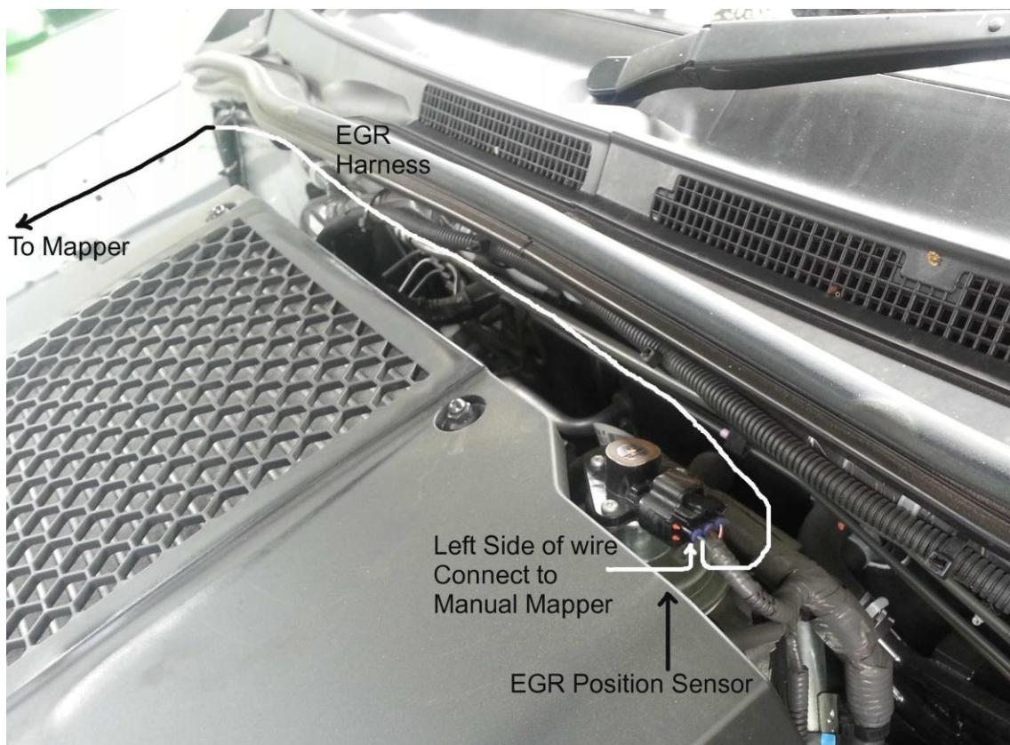
Picture of EGR Valve Position Sensor.
