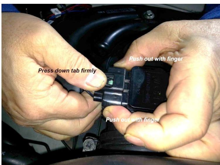
4... Connect Manual Mapper to MAF sensor on top of the air filter box by pushing the connector firmly until you feel "click".
