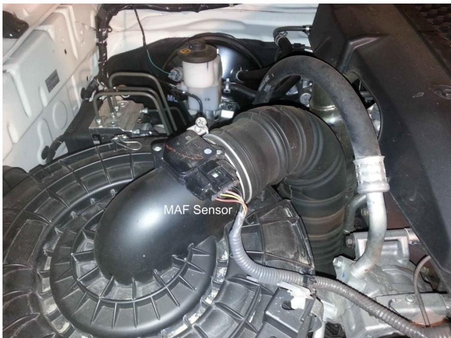
3... Disconnect the MAF sensor plug from its body. Press down the plastic locking tab on the plug, then pull out by holding the plug (Do Not pull by wire).
